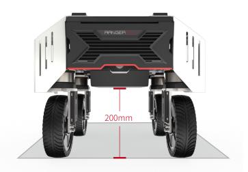
As a UGV with superb flexibility and performance, Ranger Mini combines the obstacle-climbing ability of SCOUT series with the high load capacity and long battery life of HUNTER series. Thanks to AgileX's technical heritage in motion control, it can easily operate in both indoor and outdoor environments. Swing arm suspension and higher ground clearance bring a fresh movement experience for indoor and outdoor work.
